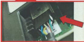
Unplug LVDS plug from board monitor and insert in LVDS IN female of the interface. Insert the plug with the white point above the middle pin of 10-Pin LVDS cable of interface into LVDS OUT female of interface, white point of plug has to show to white point of interface housing.
