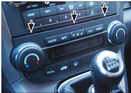
2. Unclip the air condition control unit and remove it
