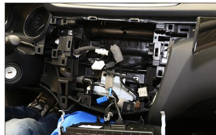
7. Dash board after removal of OEM head unit
