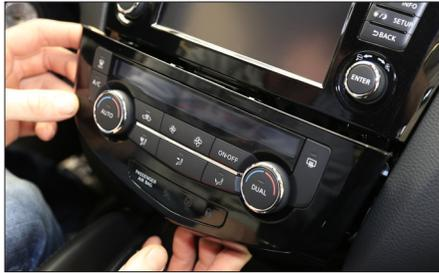
1. Unclip air condition control unit under OEM head unit
