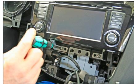
5. Remove all screws of OEM head unit
