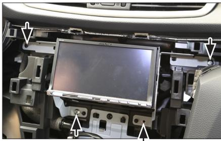
9. Connect all required circuit points. Place Double-DIN head unit on dash board
