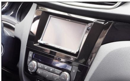
10. Put clips on the rear side of fascia plate. Place fascia plate on dash board
