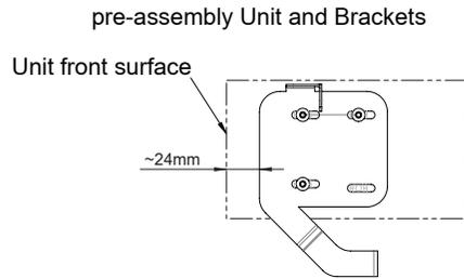
8. Mount mounting brackets with flat headed screws to Double-DIN head unit
