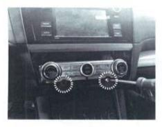
Unscrew the two screws shown in the picture and remove the clima controls panel.
