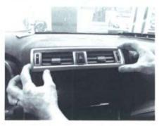
Carefully remove the air vents panel.
