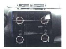
Unscrew the four screws of the original OEM shown in the picture and remove it.
