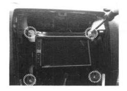
Mount the unit with the screws and verify the proper functioning of the system.
