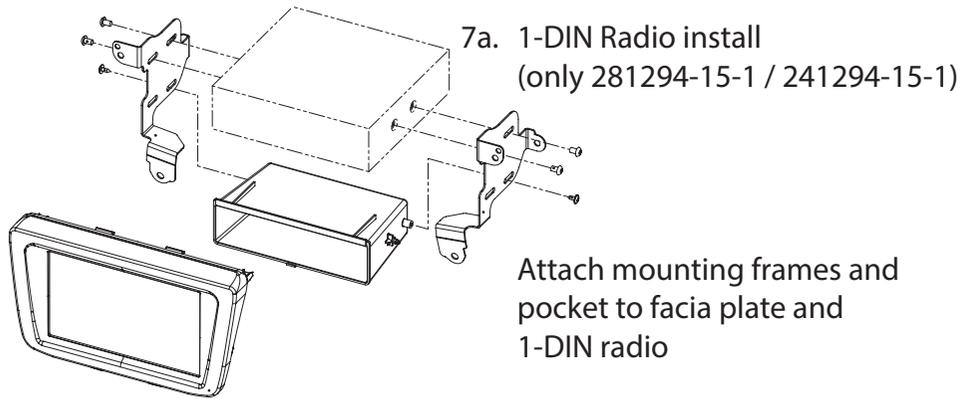
Attach mounting frames and pocket to facia plate and 1-DIN radio
